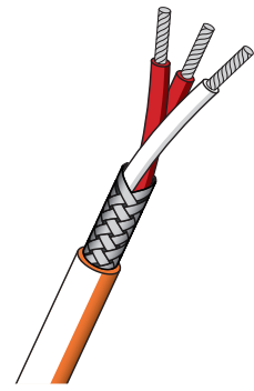
PFA Insulated with Metal Braid Cores of stranded copper conductors. Cores PFA insulated. Cores bunched together. Nickel plated copper wire braided. PFA sheathed overall. Orange outer sheath (also available with a black outer, please suffix order code with a 'B' e.g. RT37B).
