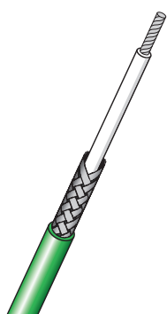
PFA Insulated Coaxial Style One pair of stranded conductors. Negative leg PFA insulated, positive leg wire braided in a coaxial style. PFA sheathed.
